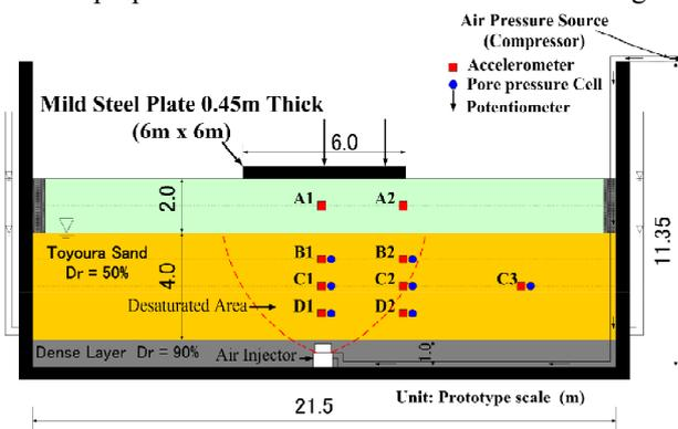
Fig 2. Desaturated Centrifuge model at 50g
