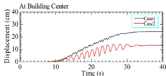
Fig 4. Vertical settlement in saturated and desaturated model at same location
