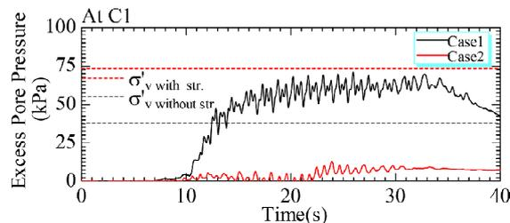
Fig 3. Excess pore pressure in saturated and desaturated model at same location
