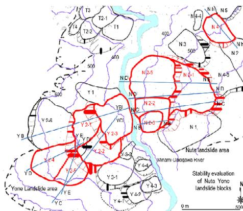
Fig 1. Identification of sliding blocks at Nuta-Yone landslides as per SABO report (2007).
