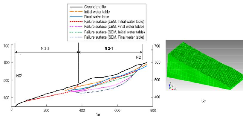
Fig 2. Slope model: (a) slope profile with water table positions and failure surfaces; (b) hexahedral discretization.
