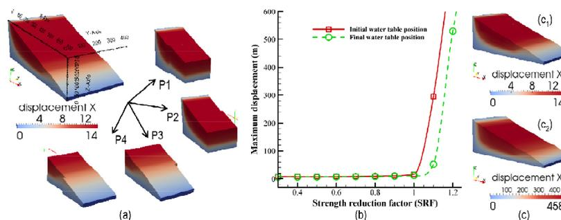
Fig 3. SEM Modeling: (a) domain decomposition; (b) displacement (m) vs. SRF; (c) displacement field at final water table positions (c1: at SRF 1.1; c2: at SRF 1.2) showing a fairly good results as compared with existing LEM.
